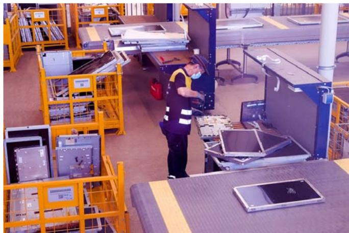
*Flat screen displayed under manual handling for dismantlement*
