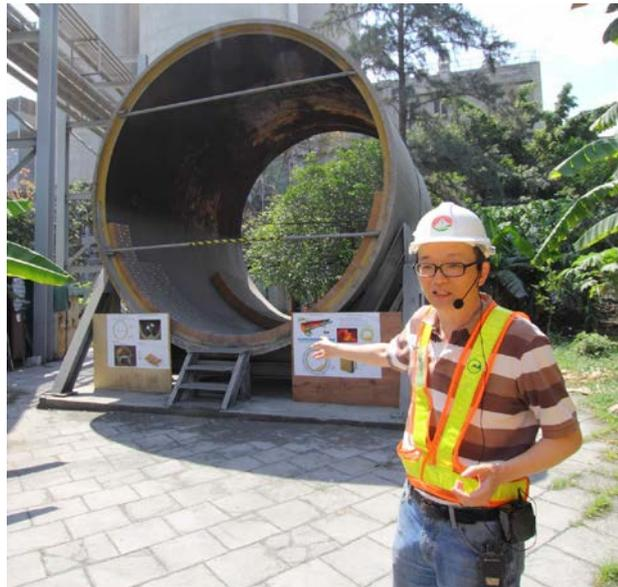
Section of Kiln Shell for demonstration and training of refractory lining
