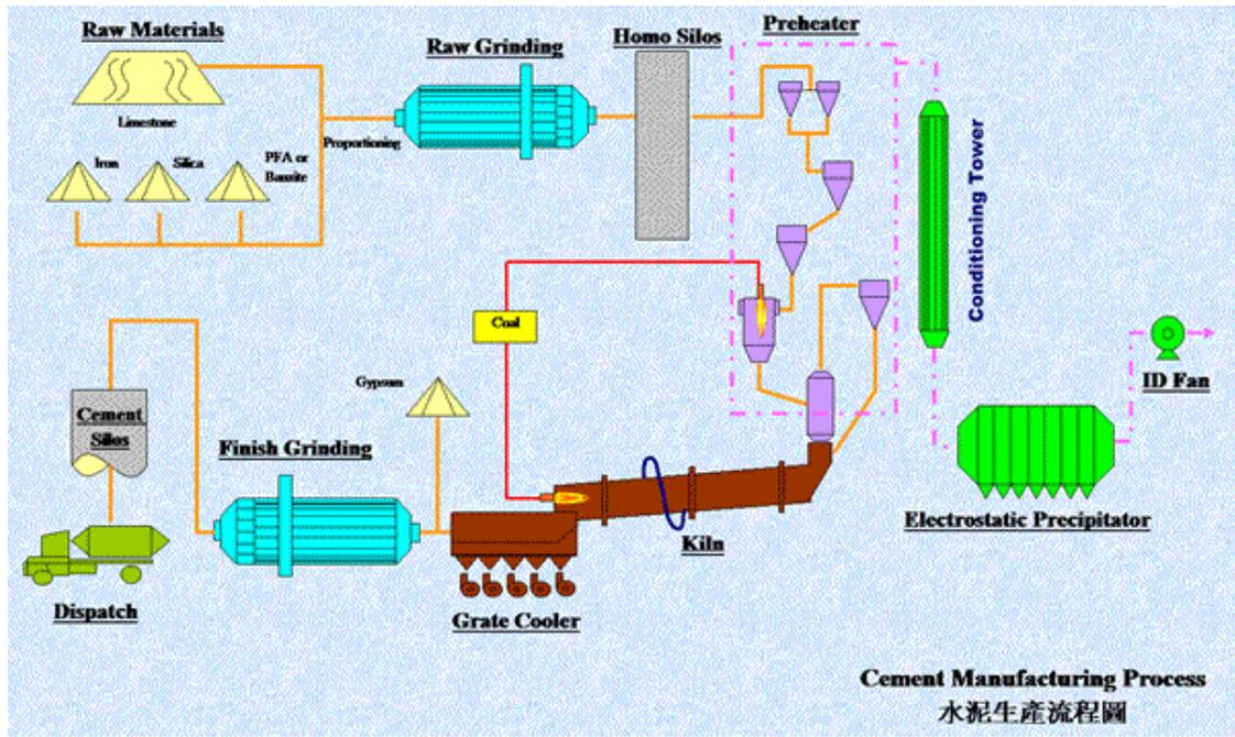
Cement manufacturing flow schematic
