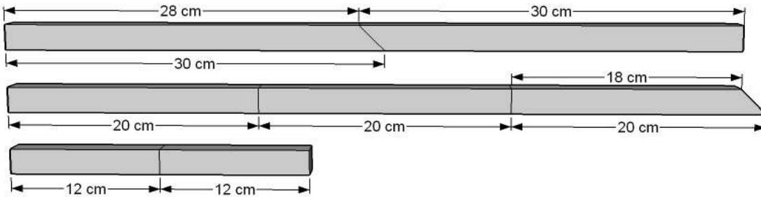
1. Cut the wood to the following lengths using the hacksaw: 3 x 200mm, 2 x 300mm, 2 x 120mm.
