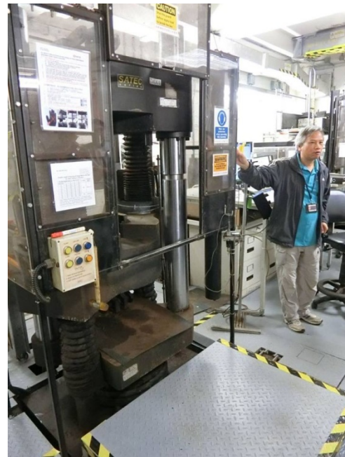
INSTRON testing machine for steel bar tensile strength tests
