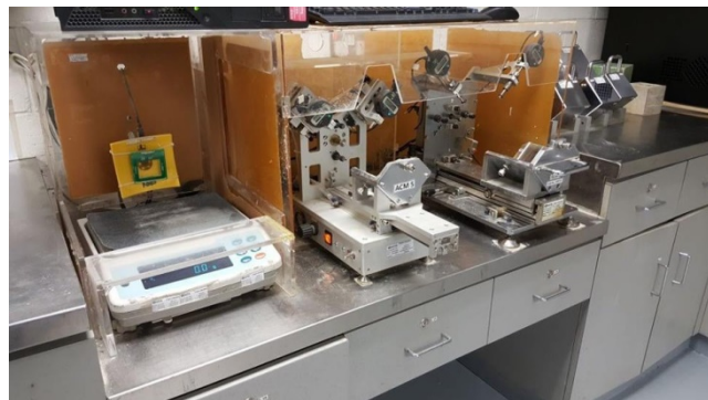
Automated dimension measurers and jigs for concrete cubes
