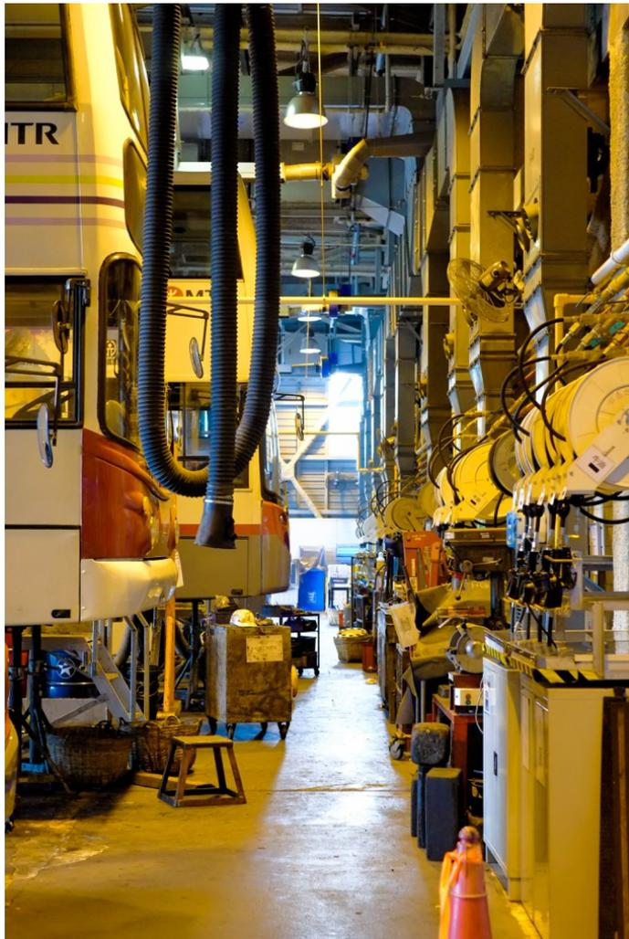
TPBMC provides Preventive Maintenance (PM) and Corrective Maintenance (CM) to MTR buses, overhaul to components and equipment and the said statutory Annual Vehicle Examination, Certificate of Roadworthiness (COR) to the MTR bus fleet. While COR is an annual undertaking for certifying the fitness of the vehicle, every bus is subject to overall visual check in Monthly Inspection and more in-depth component condition inspection, such as brake soundness, in Minor Dock between CORs.
