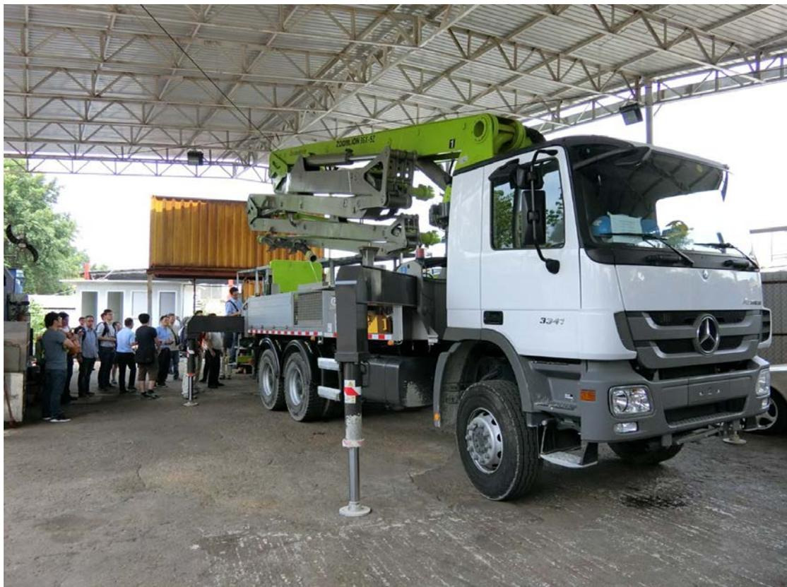
*A Zoomlion-made concrete pump mounted on a Mercedes Benz Actros 3347 truck*
