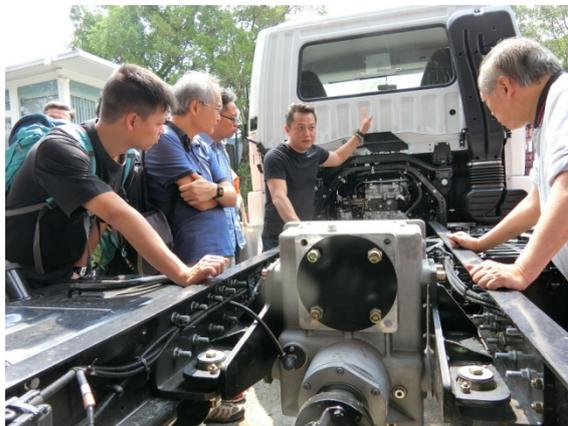
*Power Take-Off between the truck gearbox and differential gear on the rear axle to offtake power to the hydraulic pump*
