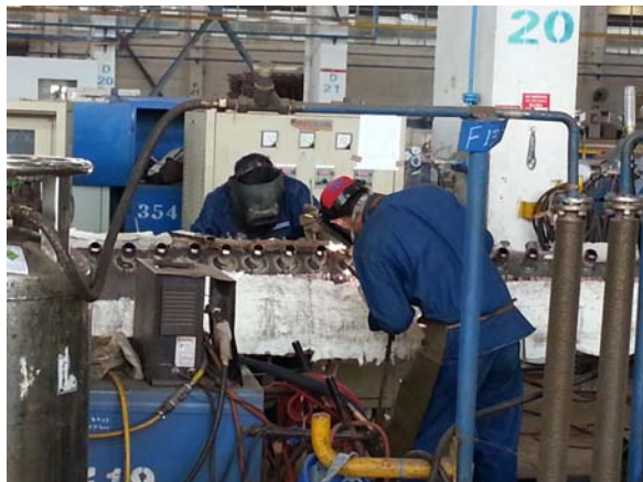
T23-made studs welded on P91 Header for Duke Energy project [W.H. Tsang]
