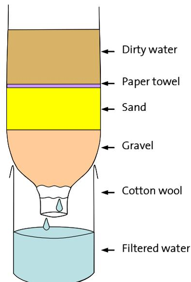
You have now constructed your filter and are nearly ready to test it. All you need to do is stand the filter (with the cotton wool at the bottom!) on top of the beaker.
